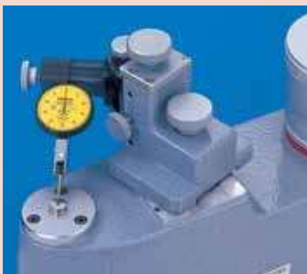
Calibrating test indicator
