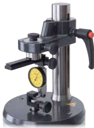
Using test indicator attachment set (02ASK000)
