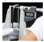
• Equipped with Ratchet Stop for constant measuring force.
